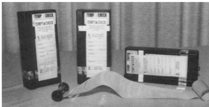
**Figure 14** Analog disposable recording temperature monitors which use a battery powered motor to pull a strip chart. The chart is obtained by breaking open the recorder box.
